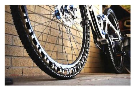
Flat bicycle tires could be a thing of the past thanks to <u>BriTek</u>'s amazin Energy Return Wheel. Whereas most bike tires regulate tire firmness with air pressure, with the Energy Return Wheel one simply adjusts the tension of the rubber that is stretched around a 29-inch <u>carbon fiber</u> wheel.
