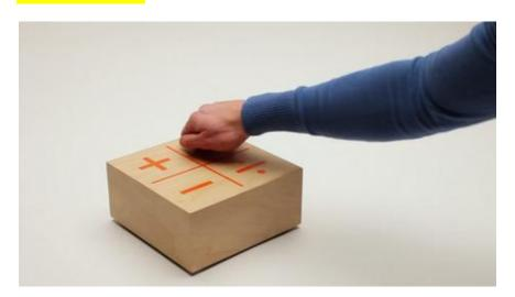
Created by Khalil Klouche and aimed at small children, Knock Knock is a playful calculator which allows calculation on the wood surface by knocking and will give back the answer using the same knocking tone. Components include <a href="Arduino">Arduino</a> board, contact microphones and solenoids.
