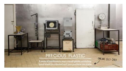
Hakken's <u>Precious Plastic</u> recycling system consists of a plastic shredder, extruder, injection moulder and rotation moulder, which have been adapted from industrial models to be more user-friendly. Hakkens intends to make the design available online so that people can set up their own workshops, recycling and producing plastic products locally, while improving upon the design in a crowd sourced way.
